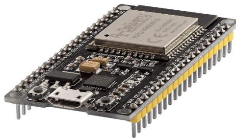
Figure 1. ESP32 microcontroller module used for signal processing, connectivity, and real-time data transmission.
