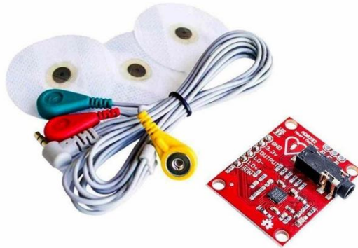
Figure 2. AD8232 ECG analog front-end module used for low-noise biopotential acquisition and real-time filtering of single-lead ECG signals.
