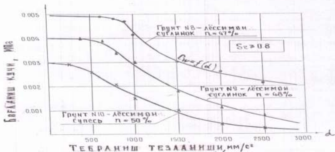
Figure 3. The dependence of the change in the binding force of a naturally soaked lucid grunt on the acceleration of vibration
