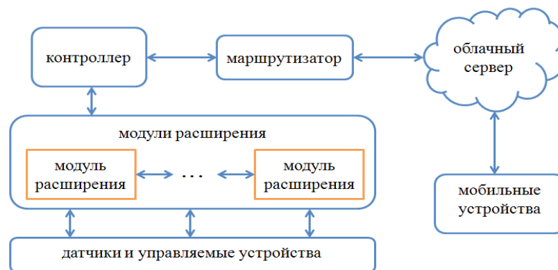
Rice. 2. Scheme of technical support for an intelligent industrial building with remote control function via the Internet
